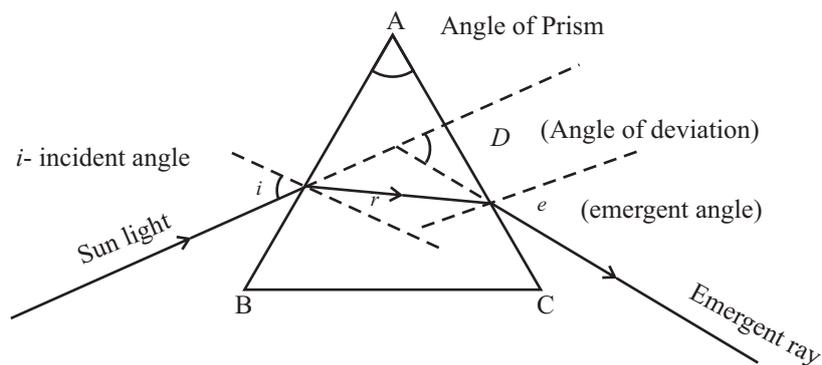
Angle of Deviation (D) The angle between the incident ray and emergent ray.
