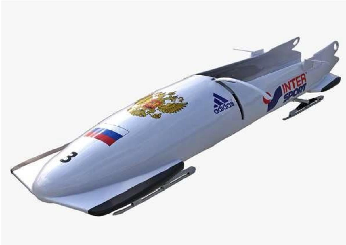
The maximum weight of a sleigh including the crews is 630kg (for four -man), 390kg (for two-man) and 340kg (for two-woman) including the additional metal weights. The Bobsleighs are designed as light as it could be to ensure dynamic movement of the crews during the turns of the course.
