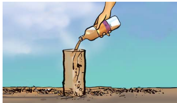
Fig. 9.5 Measuring rate of percolation
