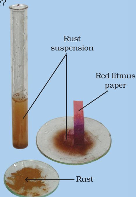
**Fig. 4.3 :** Testing the nature of rust
