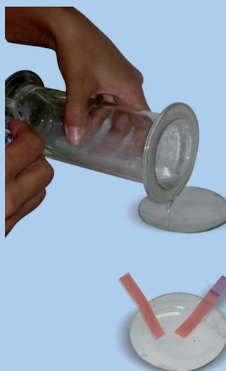
Fig. 4.4 (b) : Testing of solution with litmus papers
