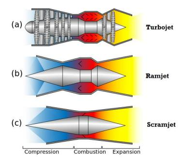
All jet engines and gas turbines work in broadly the same way. Hence they all share five key components: an inlet, a compressor, a combustion chamber, and a turbine (arranged in exactly that sequence) with a driveshaft running through them. Even though they have similarities, jet engines differ in their extra components. The main types of Jet engines based on how air is compressed in the engine are as below:
