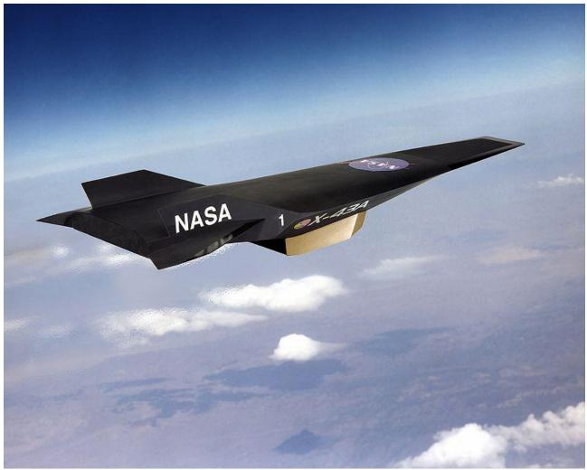
To make it simple, a scramjet is a *supersonic combusting ramjet*). This is a variant of a ramjet jet engine in which combustion takes place in supersonic airflow.
