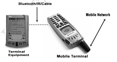
In order to take advantage of the new GPRS services, we need new GPRS enabled handsets. There are three different classes of GPRS terminal equipments:
