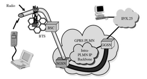
The public packet data network is only concerned that the address belongs to a specific GGSN. The GGSN hides the mobility of the station from the rest of the packet data network and from computers connected to the public packet data network.
