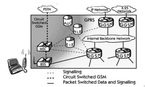
GPRS attempts to reuse the existing GSM network elements as much as possible, but to effectively build a packet-based mobile cellular network, some new network elements, interfaces, and protocols for handling packet traffic are required.
