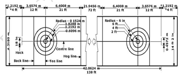
A back line of 1.83m is drawn at the back of the house. It is parallel to tee **line** which is drawn bearing a length of 4.3-4.75 m. A line that passes exactly through the center of the sheet is known as **center line**. **Target house** is present at the intersection of this tee line and center line. Apart from the central circle, three other circles are also printed with different colors.
