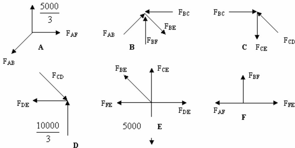
Forces at various joints of the truss in figure
