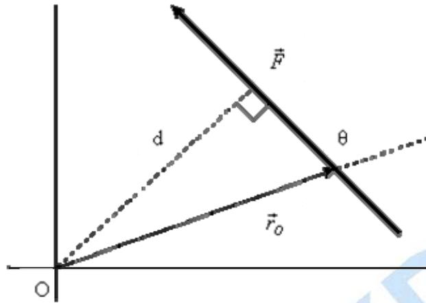
Torque is equal to the product of the magnitude of the force and its perpendicular distance  $d$  from  $O$
