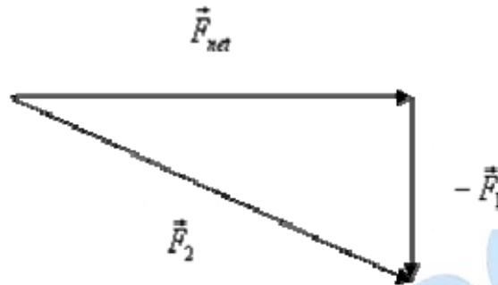
*Finding force applied by a person when the net force and that applied by one of the persons is given.*
