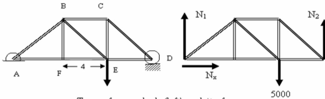
Truss of example 1 (left) and its free body diagram (right)
