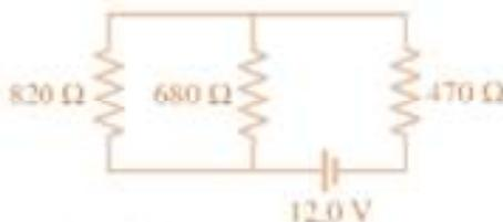
Find the equivalent resistance, Current & voltage in each resistor
